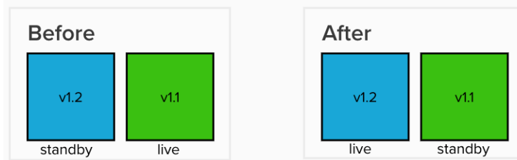
Figure 11.9 – Blue/green deployment release of a new version
