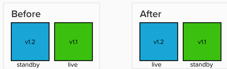
Figure 6.1 – Blue/green deployment: environment switch
