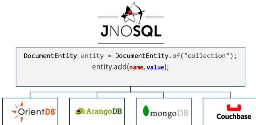
Figure 6.2: NoSQL databases – document type with a single API
