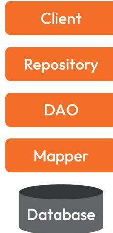
Figure 4.5 – Up-front design using repository pattern
