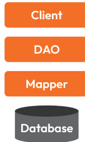
Figure 4.4 – Upfront design using DAO pattern brings even more abstraction to the database integration
