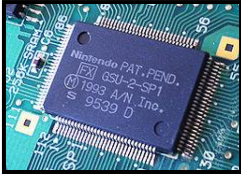
Fig. 5.31 Chip " Super FX " (Cartucho Super Nintendo )
