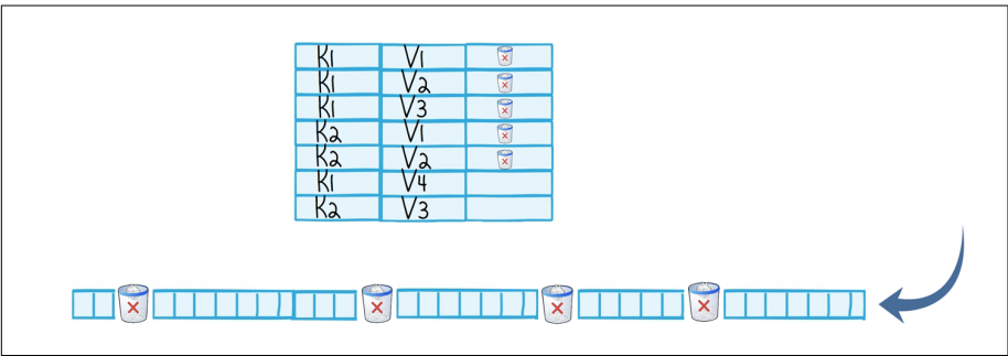
Figure 4-5. In a compacted topic, superseded messages that share the same key are removed. So, in this example, for key K2, messages V2 and V1 would eventually be compacted as they are superseded by V3.
